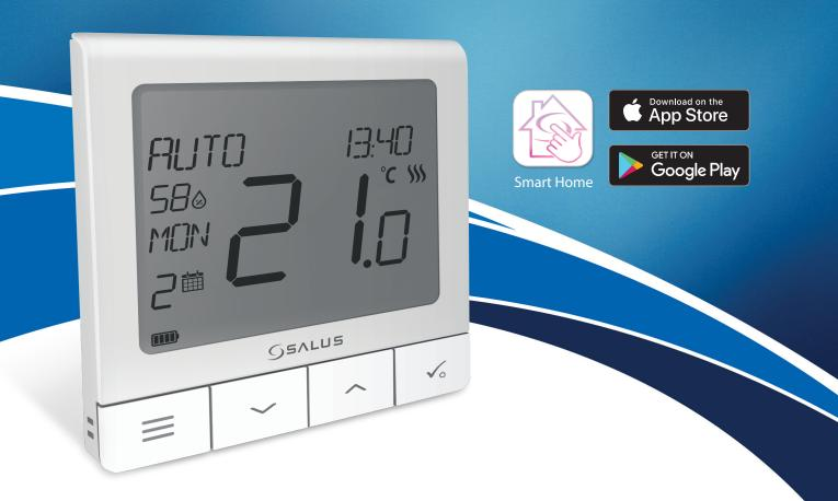
The NEW Quantum SQ610 thermostat is the latest innovative addition to the SALUS portfolio. This sleek and stylish thermostat is the slimmest on the market at only 10mm thick\*. It is powered by 230V. The SQ610 is a truly unique thermostat, allowing a choice of hard wired connectivity or RF communication via 2.4 GHz, giving you easy connection to your SALUS Smart Home controls.
